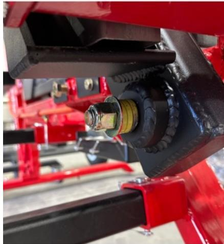
The main dash bolt nut should not loosen or move, however occasionally check to be sure that it is properly in place with full compression on the yellow spring.
