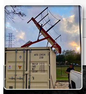
FireVent's Portable Units are designed to be easy to set up and take down and move from location to location. These units are able to go from a flat position to a 12/12 pitch. There are currently two sizes available; 8ft x 12ft and 10ft x 16ft.
